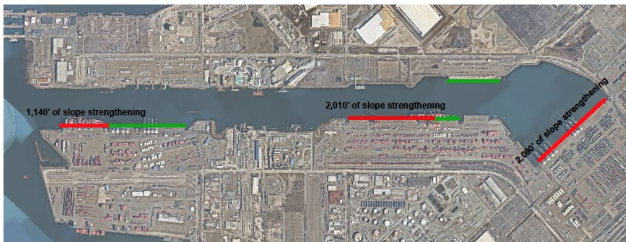
Figure 5-2. Anticipated Slope Strengthening by Facility for Depth Below -54 MLLW.
